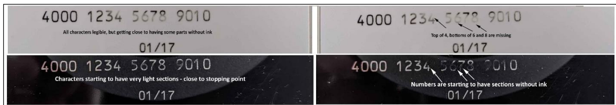
Figure 17 – Before(left) and after(right) wear-through occurs
