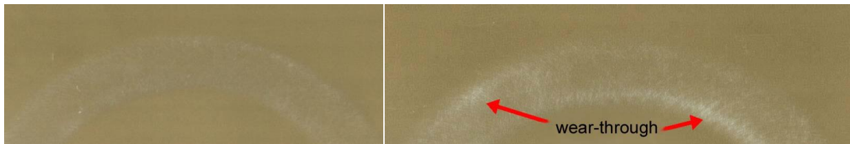
Figure 16 – Before(left) and after(right) wear-through occurs
